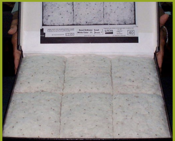
Figura 10. Padrões físicos universais do algodão americano Upland – "Good Middling White Color (11), Leaf Grade (1)" e "Good Ordinary White Color (71), Leaf Grade (7)" (Foto: J. J. de Lima)
